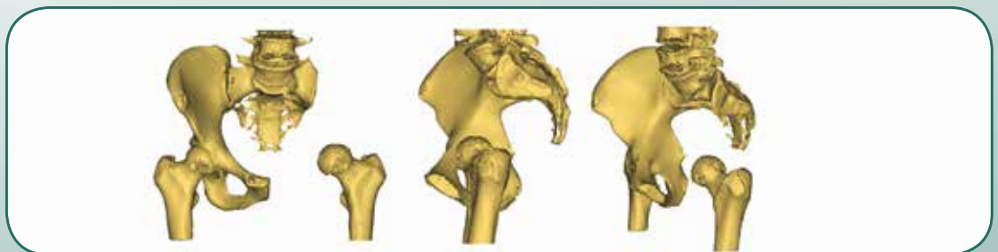
simulated situation after resection: anterior, lateral and isometric view
