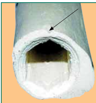
Fig. 1: Hexagonal implant bed in a bone model
